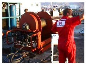
Above Left – 10 Tonne Subsea winch installed on davit for the EM tether repair (2010 - see page 4).
