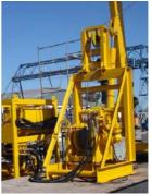
**Above Left - 12 Tonne High Speed Tool Deployment Winch Stolt Offshore (2000 – 2001)** Winch with 140 kW power-pack– Designed for 1,500 meters of 26mm SWR and used by Stolt Offshore in deep water oil field installation (Girrasol Field) activities off Angola.
