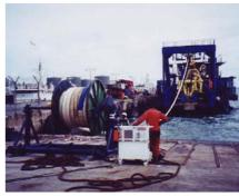
**Above Left**: Hydraulically powered reel for sub sea hydraulic hose umbilicals. **Centre**: Hydraulically powered reel with rim drive pneumatic wheel **Right**: Hydraulically powered reeling system for varying drum sizes
