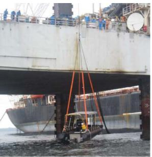
**Above** Rhino 9.5 m with 280 hp inboard diesel Volvo Penta Z drive for Perenco 2008 on sea trials in Cape Town (left) and in use being lifted onto jack up rig near Douala Cameroon.
