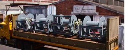
**Set of 4 mooring winches (2002) for the Hydro Dive DSV "HD Commander" in Nigeria.** Each winch carries 1,500m of 28mm SWR and has a bare drum pull capacity of 30 tonnes. The winches are driven via a 110 kNm final drive planetary gearbox mounted inside the winch drum to minimise the space requirements. Winches are horse-power controlled for power efficiency. The two bow winches are fitted with automatic spooling.
