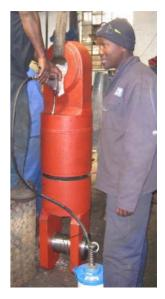
**Above** 300 Te linear winch supplied to Leighton India for onshore pipe-pull during test loading. Balancing sheave in foreground. **Above right** 300 Te swivel supplied with winch.
