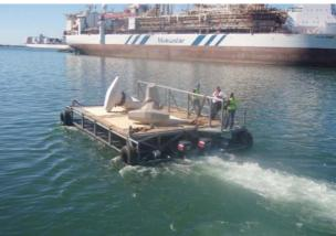
Wale Marine were commissioned to design a light-weight, low draught self propelled transport barge for transporting dollosse and construction equipment from a supply vessel to the Calshot harbour. The barge was fabricated from HDPE pontoons with a steel space frame superstructure.
