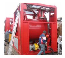
**Above Left**. Two pneumatically powered umbilical reels fabricated in Cape Town and supplied via Wale Marine Australia (no longer operating) for Well Ops in Australia
